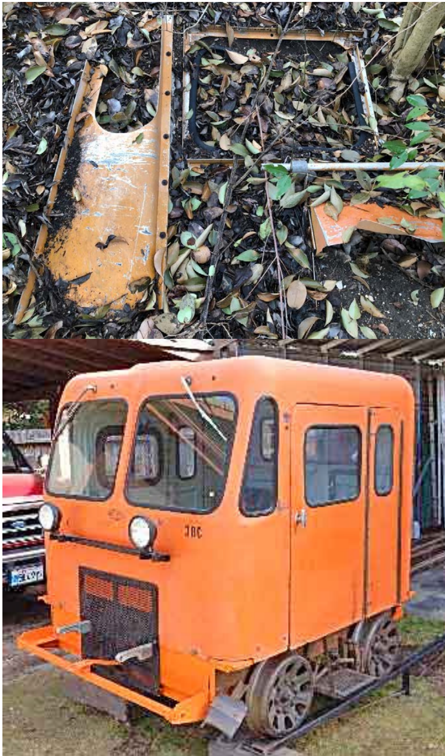
Figure 34. Site 41WM1435, Top- Remains of a railroad train speeder car (also known as track maintenance or inspection car) found on the west slope of the railroad embankment. Bottom- example of a complete speeder car (North American Railcar Operators Association 2021).
