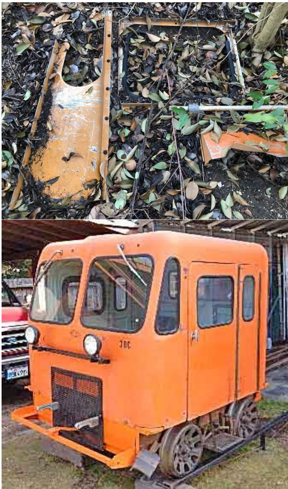
Figure 21. Site 41WM1435, Top- Remains of a railroad train speeder car (also known as track maintenance or inspection car) found on the west slope of the railroad embankment. Bottom- example of a complete speeder car (North American Railcar Operators Association 2021).
